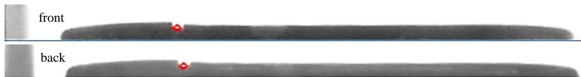
Fig. 7 The detected top edge material defects
