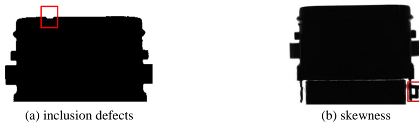
Fig. 2 Two types of side layer defects for the silicone rubber gaskets from side-view
