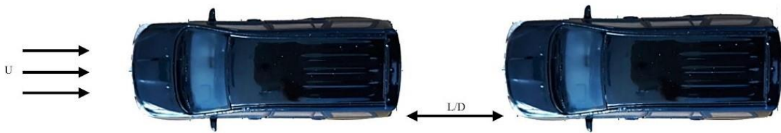
Fig. 1 The positions of the first minibus and the second minibus in a series tandem model
