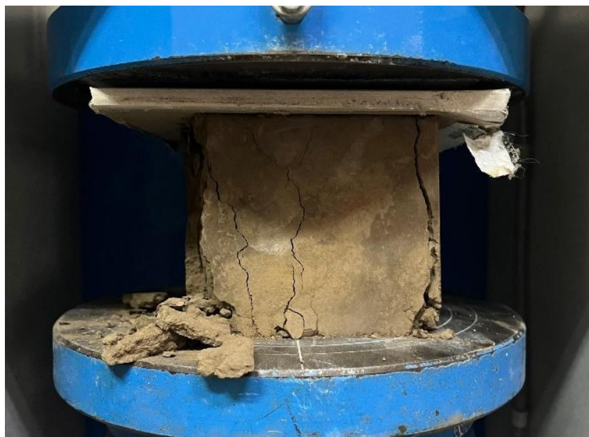
Fig. 4 Compressive strength test setup of sample
