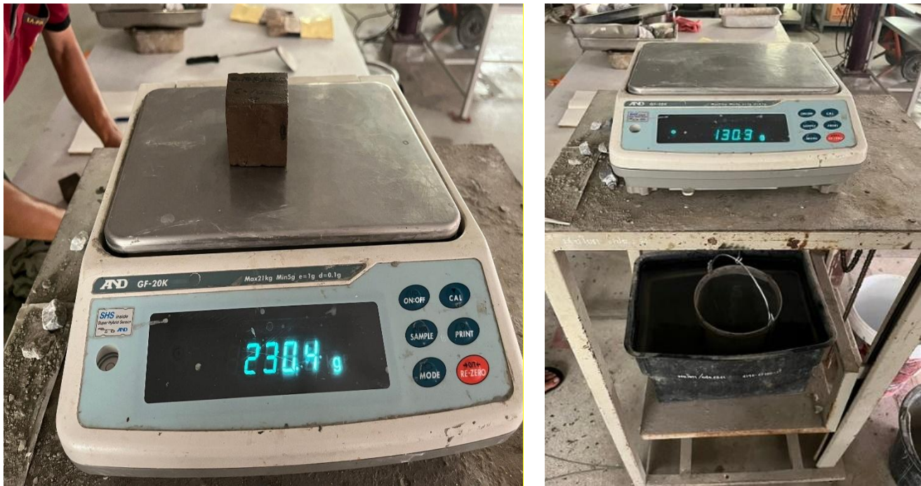
(a) Measurement of the weight of the oven-dried sample
