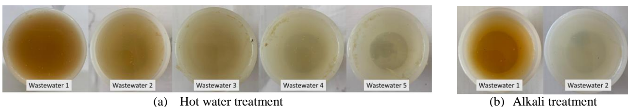
Fig. 4 Color change of the wastewater of BF in each cycle
