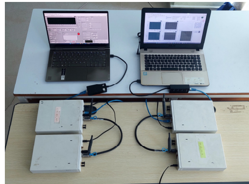
(b) Realization of MIMO-OFDM transceiver on NI-USRP
