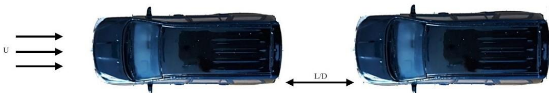
Fig. 1 The positions of the first minibus and the second minibus in a series tandem model
