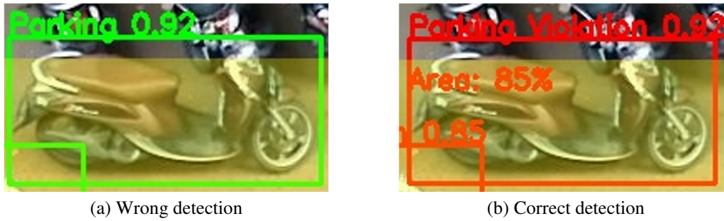
Fig. 15 Detection results without and with the application of the object area calculation method
