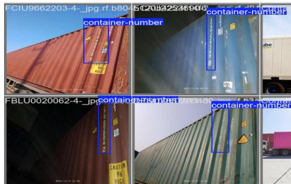
Fig. 4 The results of using YOLOv11n with the container region detection algorithm
