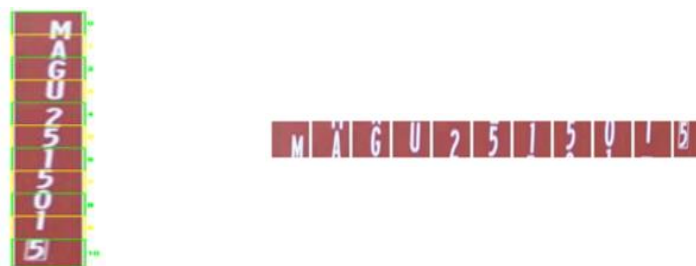
(a) Character segmentation regions (vertical layout) (b) Concatenated characters in a horizontally aligned format
