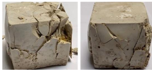
Fig. 9 Typical compressive failures of BFG (T5-UT4)
