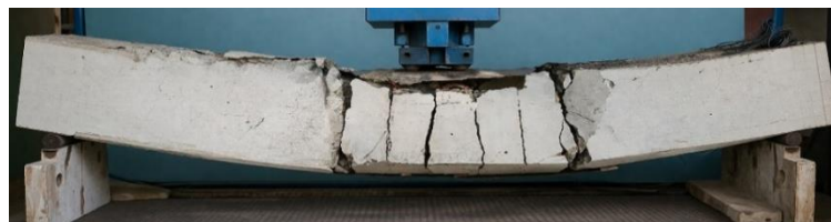
Fig. 10 Typical failure mode of steel-reinforced beam after flexural testing
