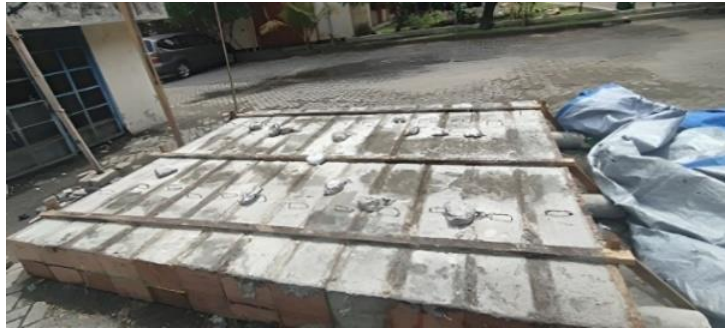
Fig. 3 Curing process of the reinforced concrete beam specimens
