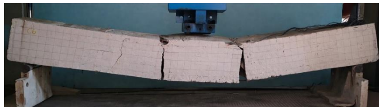
Fig. 9 Typical failure mode of GFRP-reinforced beam after flexural testing
