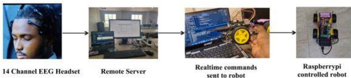
Fig. 6 Implemented BCI framework
