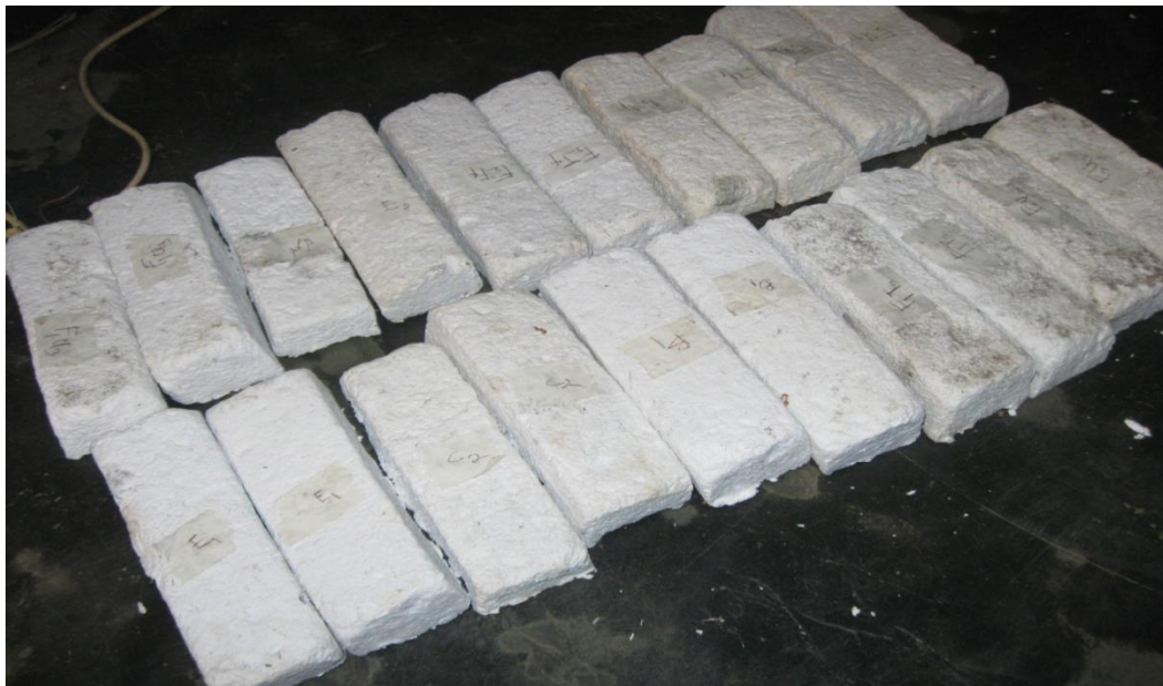
Fig. 2 Samples prepared for flexural test
