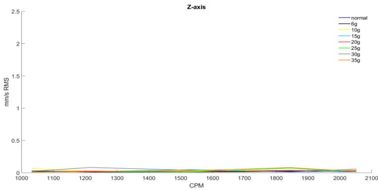
Fig. 4 Relationship between the amplitude and rotary speed along the z-axis (axial direction) (mm/s RMS – CPM)
