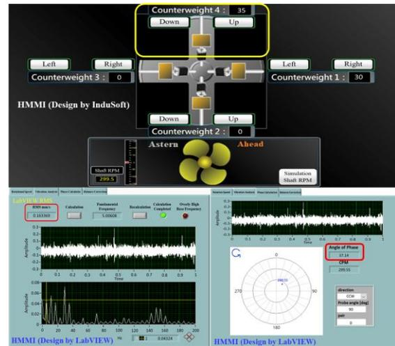
Fig. 16 Counterweight 4 moves 35 steps for system imbalance correction
