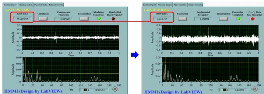
Fig. 13 RMS change with 66 g weight imbalance
