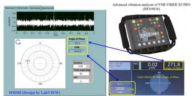
Fig. 3 Schematic of signal accuracy validation
