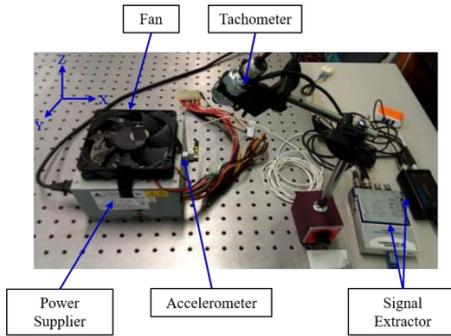
Fig. 2 The simple experimental platform designed in the preliminary phase
