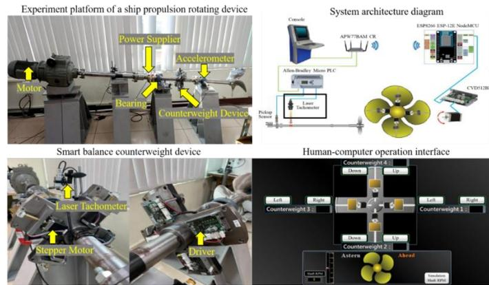
Fig. 1 Vibration monitoring and balance correction for ship propulsion rotating devices
