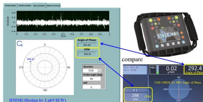
Fig. 10 Comparison of the CPM and phase angle values obtained from HMMI and VMI-VIBER X5 PRO
