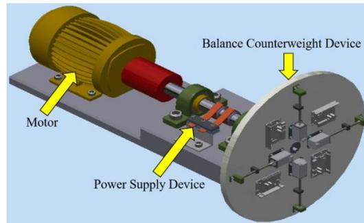
Fig. 7 Prototype of the automatic balance correction system
