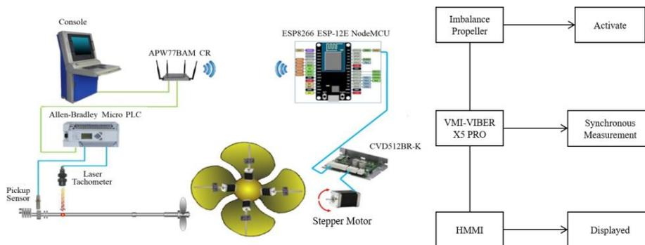
Fig. 11 System structure of the experimental simulation platform
