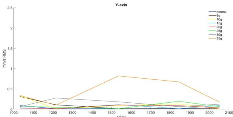
Fig. 6 Relationship between the amplitude and rotary speed along the y-axis (radially front and back) (mm/s RMS – CPM)
