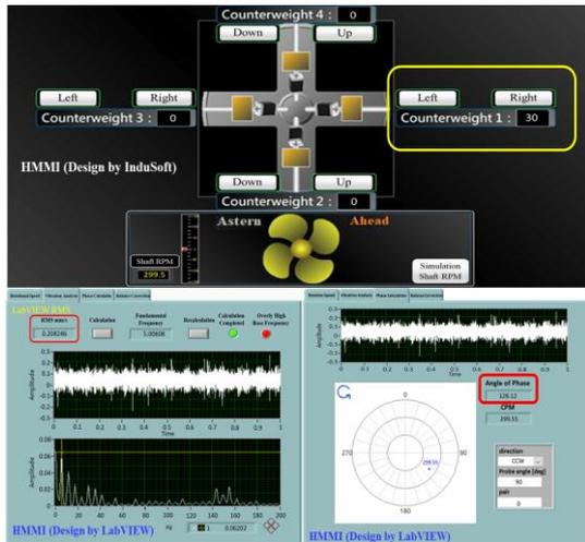
Fig. 15 Counterweight 1 moves 30 steps for system imbalance correction
