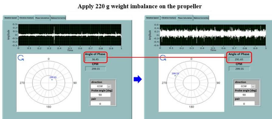
Fig. 18 Phase angle change with 220 g weight imbalance
