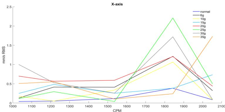
Fig. 5 Relationship between the amplitude and rotary speed along the x-axis (radially left and right) (mm/s RMS – CPM)
