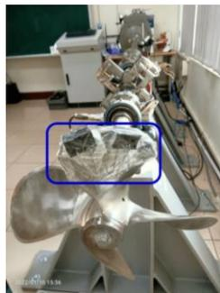
Fig. 8 Weights attached to a propeller to simulate imbalance
