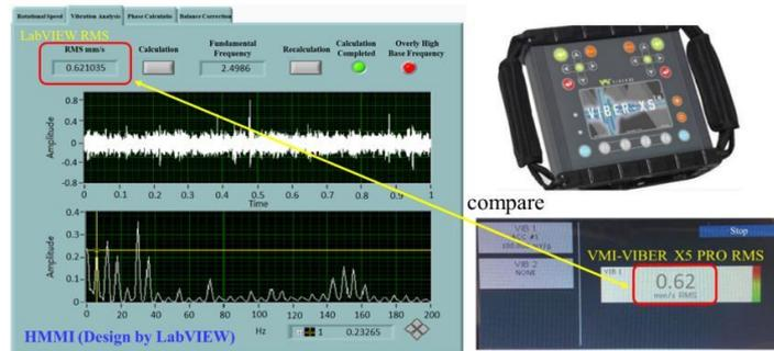
Fig. 9 Comparison of the RMS value obtained from HMMI and VMI-VIBER X5 PRO
