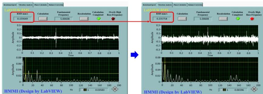
Fig. 13 RMS change with 66 g weight imbalance
