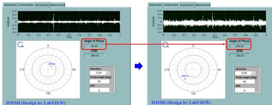
Fig. 14 Phase angle change with 66 g weight imbalance
