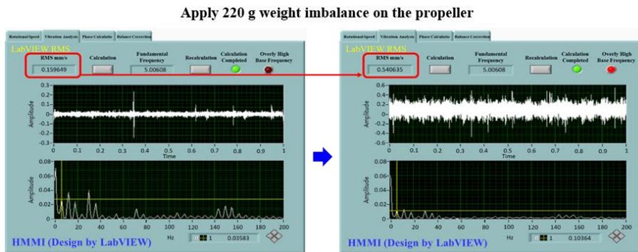
Fig. 17 RMS change with 220 g weight imbalance
