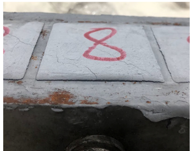
(b) High temperature (80 °C) caused the expansion
