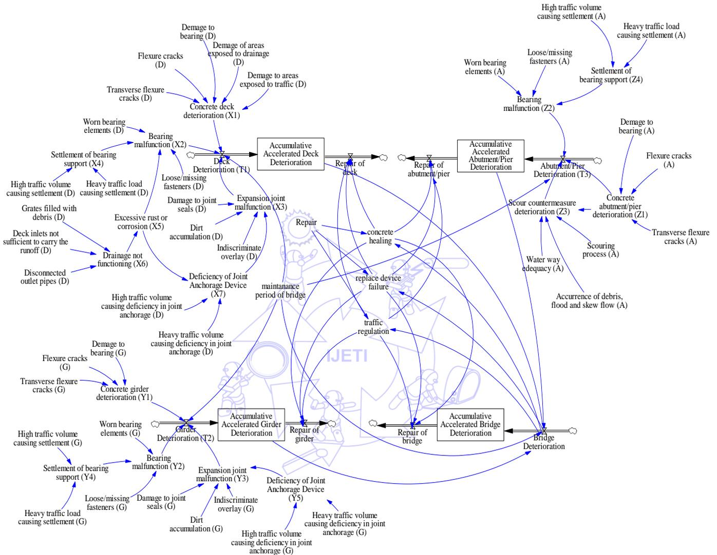
Fig. 3 SD model for bridge deterioration
