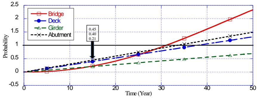
(a) Accelerated bridge and components deterioration [ $P(d)$ ,  $P(g)$ ,  $P(a)$  = preliminary probabilities]
