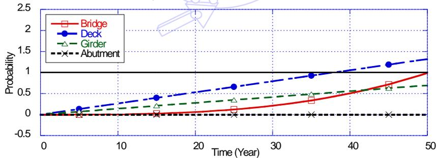
(d) Accelerated bridge and components deterioration [ $P(a) = 0$ ,  $P(d)$ ,  $P(g)$  = preliminary probabilities]
