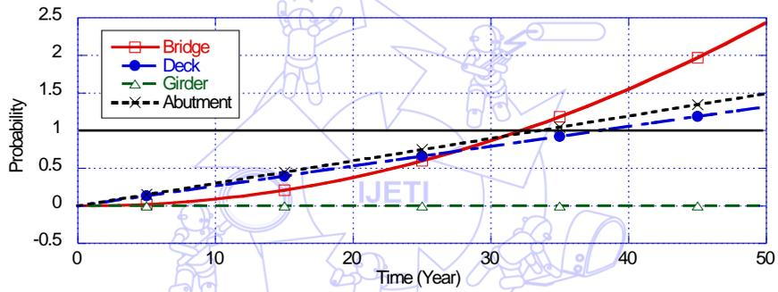
(c) Accelerated bridge and components deterioration [ $P(g) = 0$ ,  $P(d)$ ,  $P(a)$  = preliminary probabilities]
