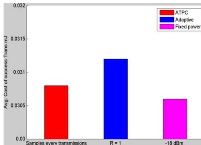
Fig. 5 University building- Comparison of the minimum cost due to different transmission strategy shows that there is hardly any difference in the average cost per successful transmission
