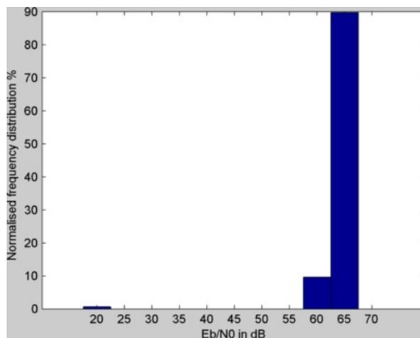
Fig. 4 The frequency distribution plot of the received  $E_b/N_0$  from data set 1 shows that occasionally the signal level has dropped by 30-40 dB, primarily due to multipath fading. Overall, the link quality has been good
