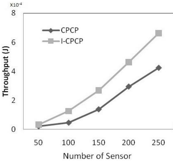
Fig. 4 Network lifetime (homogenous WSNs) achieved by proposed I-CPCP and CPCP [11] with cost  $C_{mw}$
