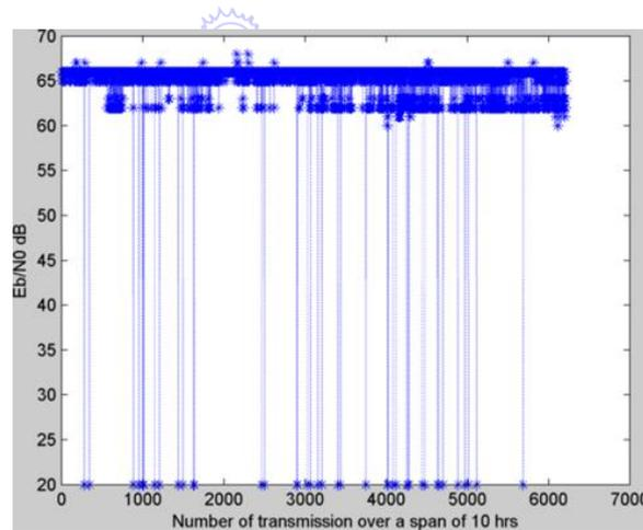
Fig. 3 The variation of the average  $E_b/N_0$  over time. Along x-axis, the numbers of transmissions are noted. The average  $E_b/N_0$  is quite high ( $>60$  dB) and occasionally dropped to 20 dB. Since the distance between the access point and the laptop is constant, the drop in the value is attributed to human movements in between and multipath effects
