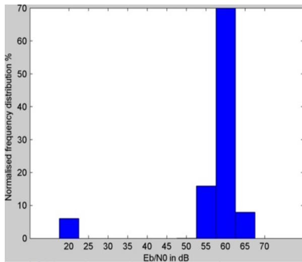
Fig. 7 The frequency distribution plot of the received  $E_b/N_0$  from University dining hall during busy hour shows the rapid fluctuation in the signal level caused by movements of people in between the transmitting sensor and receiver
