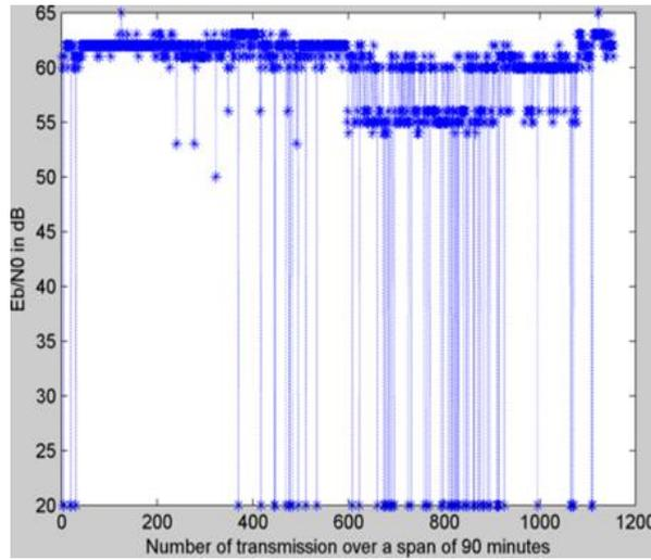
Fig. 6 The variation of the average  $E_b/N_0$  from University dining hall during busy hour between 11:30 a.m. and 1:00 p.m. The average  $E_b/N_0$  is quite high (>55 dB) and occasionally dropped to 20 dB. The busy hour period shows that the average  $E_b/N_0$  can widely fluctuate between high  $E_b/N_0$  (> 55 dB) and low  $E_b/N_0$  (~20 dB)
