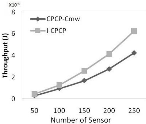
Fig. 8 Network lifetime (heterogeneous WSNs) achieved by proposed I-CPCP and CPCP [11] with cost Cmw
