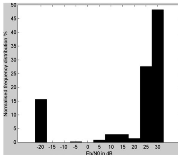
Fig. 17 Town shopping center- The frequency distribution of the  $E_b/N_0$  values during busy hour shows that the channel quality has oscillated between good and bad. In good state most of the packets will be successfully transmitted, while in bad state almost
