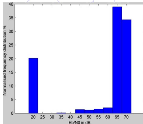
Fig. 10 The distribution plot of the received  $E_b/N_0$  from town shopping centre during busy hours between 11:30 a.m. and 1:30 p.m. shows that  $E_b/N_0$  at 20 dB is significantly high (~20%) which indicates that link quality has fluctuated frequently
