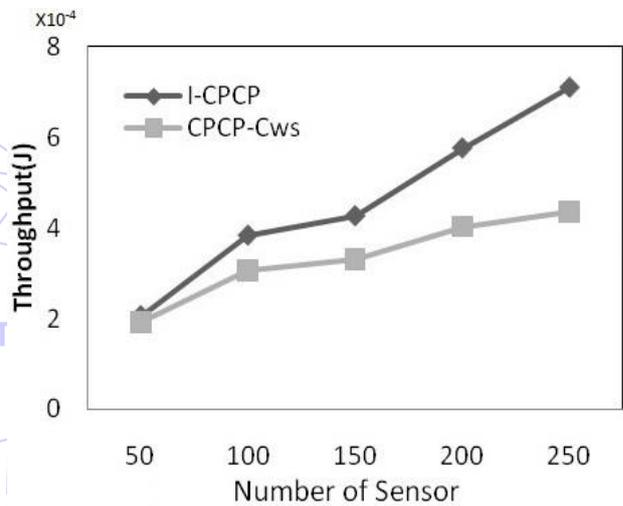
Fig. 9 Network lifetime (heterogeneous WSNs) achieved by proposed I-CPCP and CPCP [11] with cost Cws.
