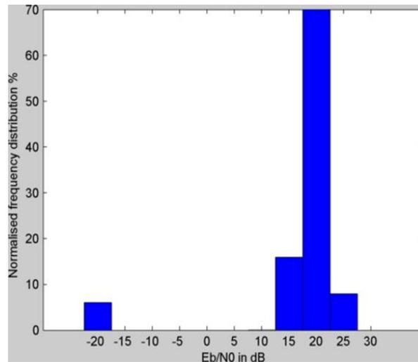
Fig. 16 University dining hall - The frequency distribution of the  $E_b/N_0$  values in during busy hour shows that the channel quality has oscillated between good and bad. In good state most of the packets will be successfully transmitted, while in bad state almost no packet transmission will be successful
