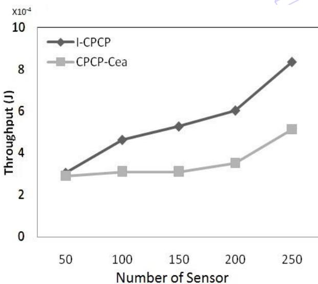
Fig. 6 Network lifetime (homogenous WSNs) achieved by proposed I-CPCP and CPCP [11] with cost  $C_{ea}$
