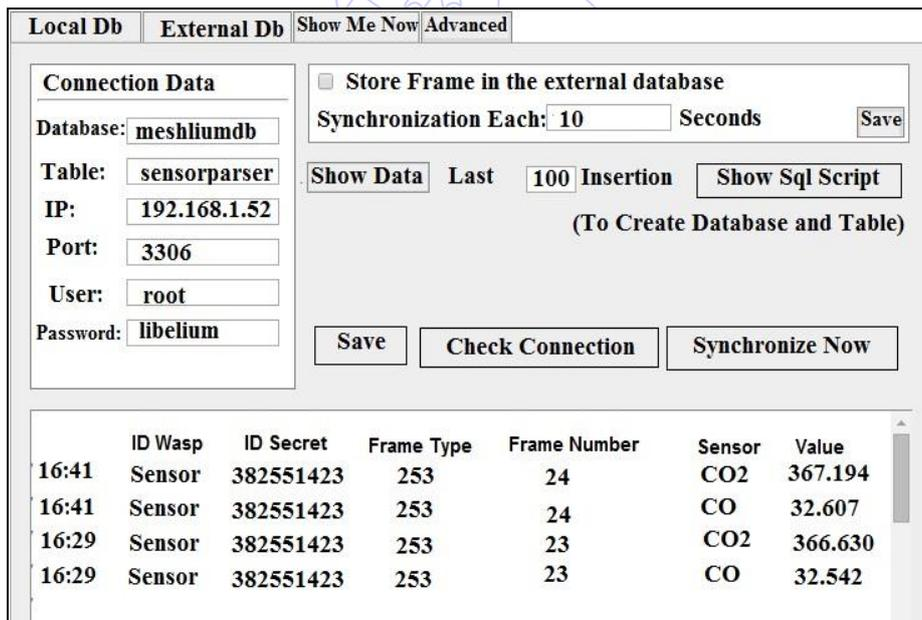
Fig. 8 External Database Synchronization
