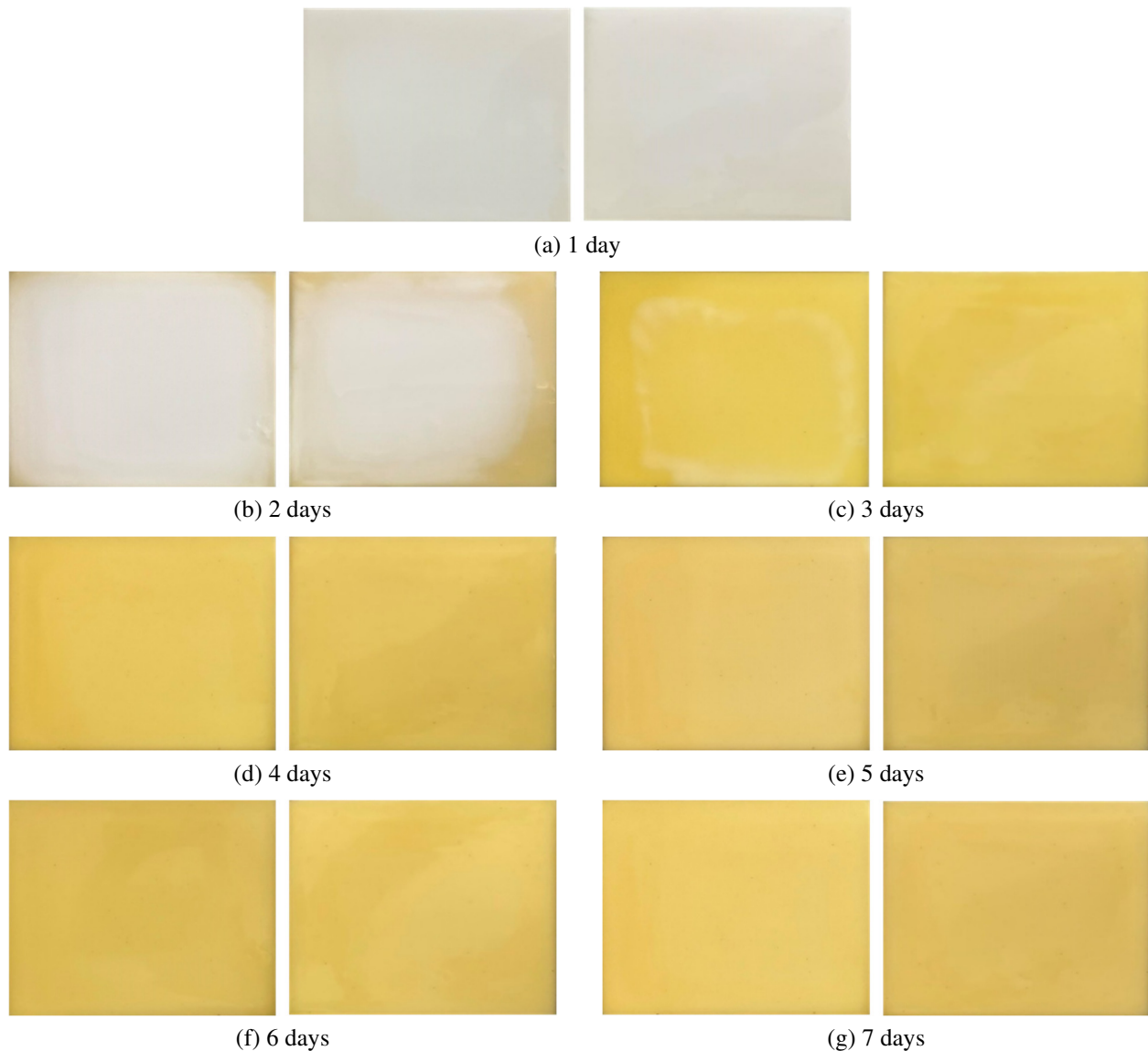
Fig. 1 The dried and cured self-repairing natural rubber sheets at 30 °C or room temperature under UV lighting
