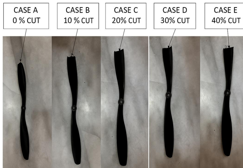
Fig. 3 Cases for Propeller 8045 Faults
