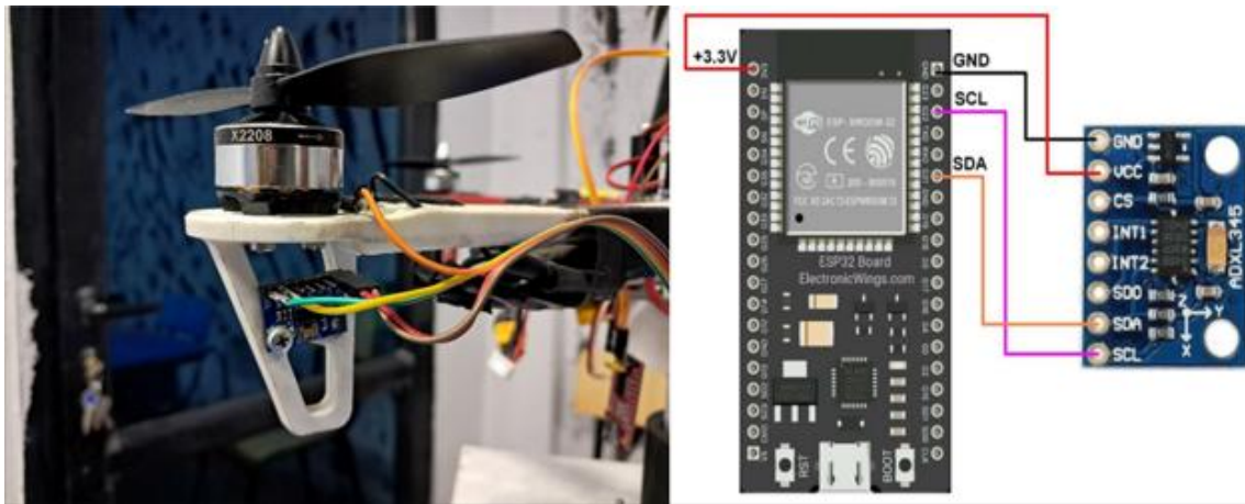
Fig. 2 Designed data acquisition and anomaly detection hardware
